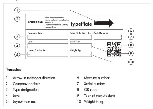
The information on the nameplate is used to identify the conveyor. The type designation is required to use the conveyor according to its intended use.
