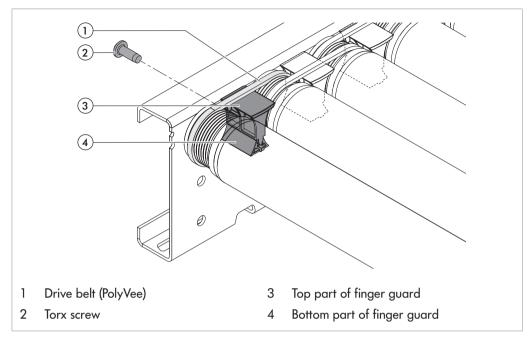
The finger guard protects against injuries as well as damage to the belt.
