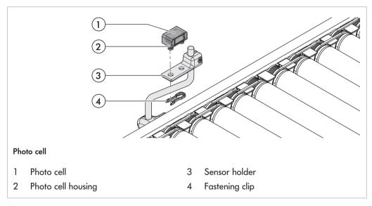
The photo cell is replaced together with the photo cell housing and the fastening clip:
