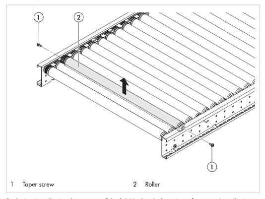
Replacing the roller is only necessary if the PolyVee heads show signs of wear or the roller is damaged.
